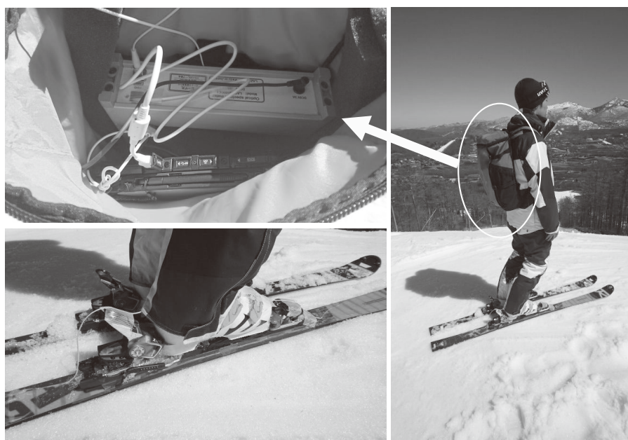
Figure 8. Conventional FBG system.
