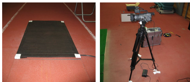
Fig. 2: The experiment equipments (left: switch mat, right: video camera).
