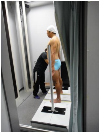
Figure 1. Measurement of 3-dimensional body geometry by a body line scanner.
